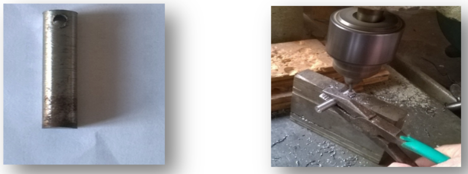
Figure 2. Preparation of the sample for the weight loss measurements
