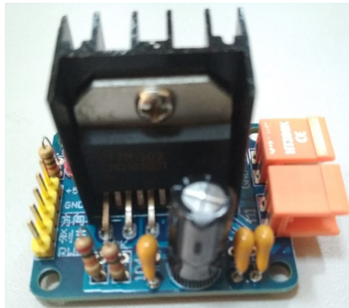
Figure 6. DC motor driver that constitutes the test setup
