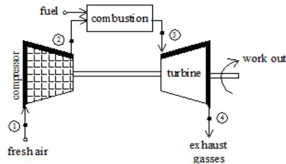
*Figure 1. Gas power plant working cycle*
