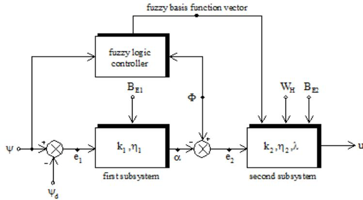
Figure 5. Structural diagram of the back stepping surge control system
