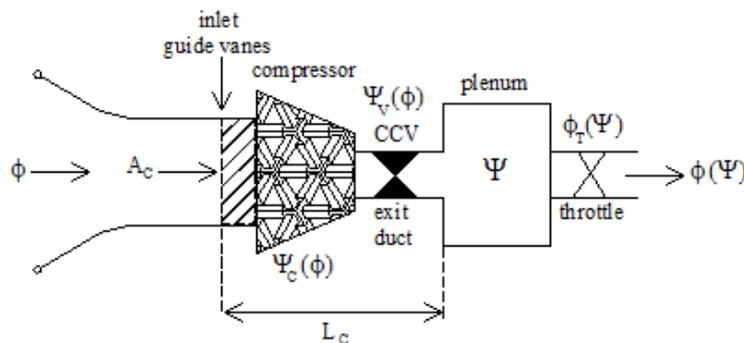
Figure 4. The structure of system compression system with valve
