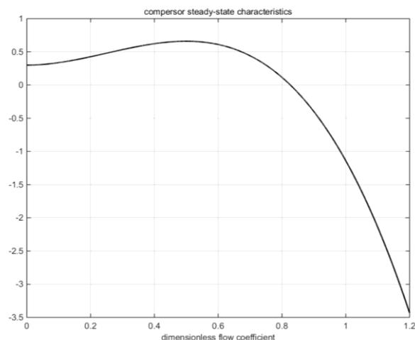
Figure 3. Permanent-state characteristic of the compressor
