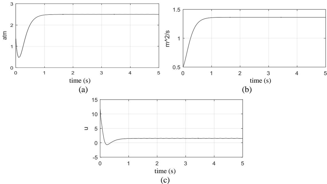
**Figure 9.** Input flow rate coefficients, output pressure and control signal with designed controller to dynamic surface method, (a) Changes in the output pressure coefficient, (b) Changes in the input flow rate coefficient and (c) Control signal
