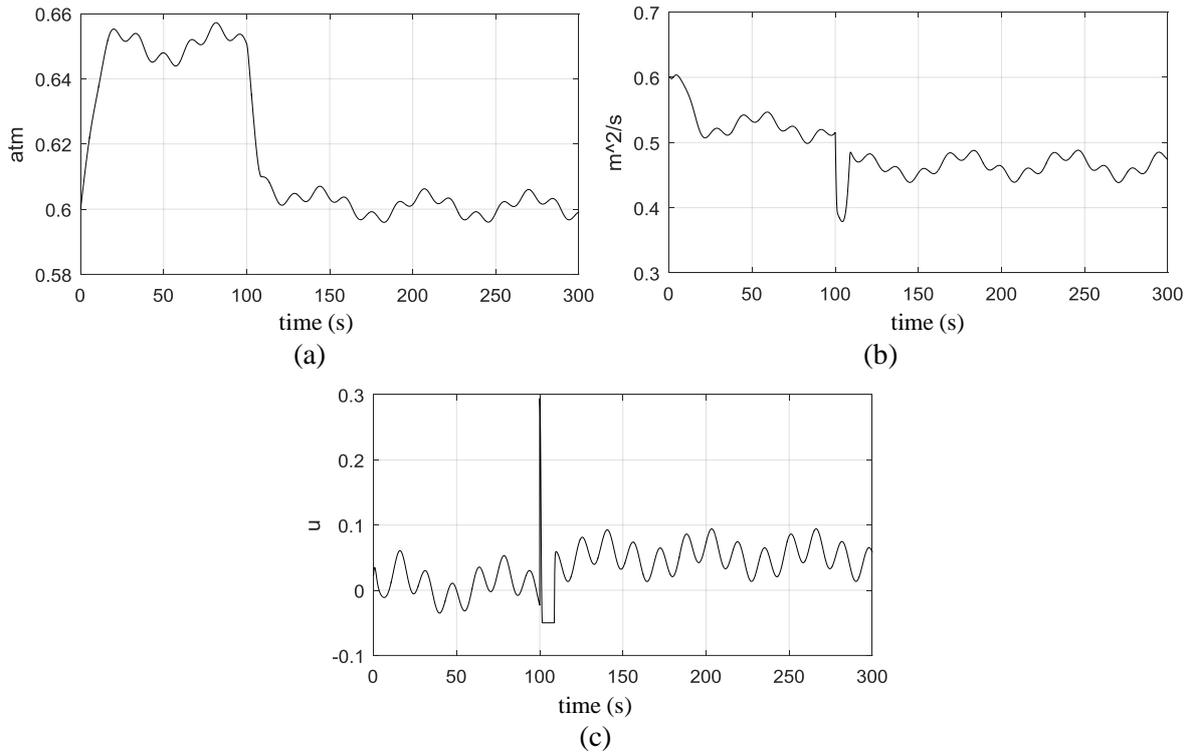
**Figure 11.** Input flow rate coefficients, output pressure and control signal with designed controller to back stepping method with environmental disturbance, a) Changes in the output pressure coefficient, b) Changes in the input flow rate coefficient and c) Control signal
