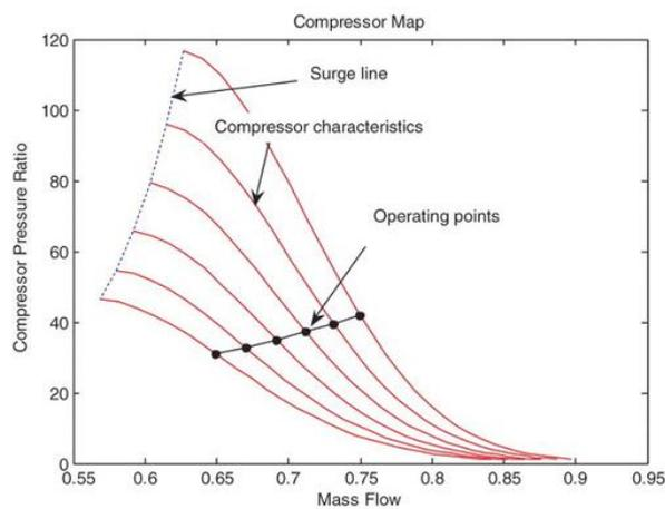
**Figure 2.** Specifying the surge line in the compressor performance diagram
