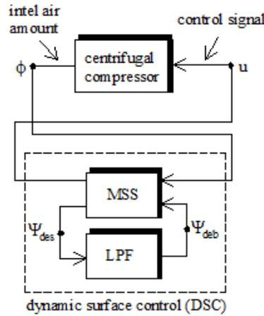
**Figure 6.** Structural diagram of the dynamic surface surge control system
