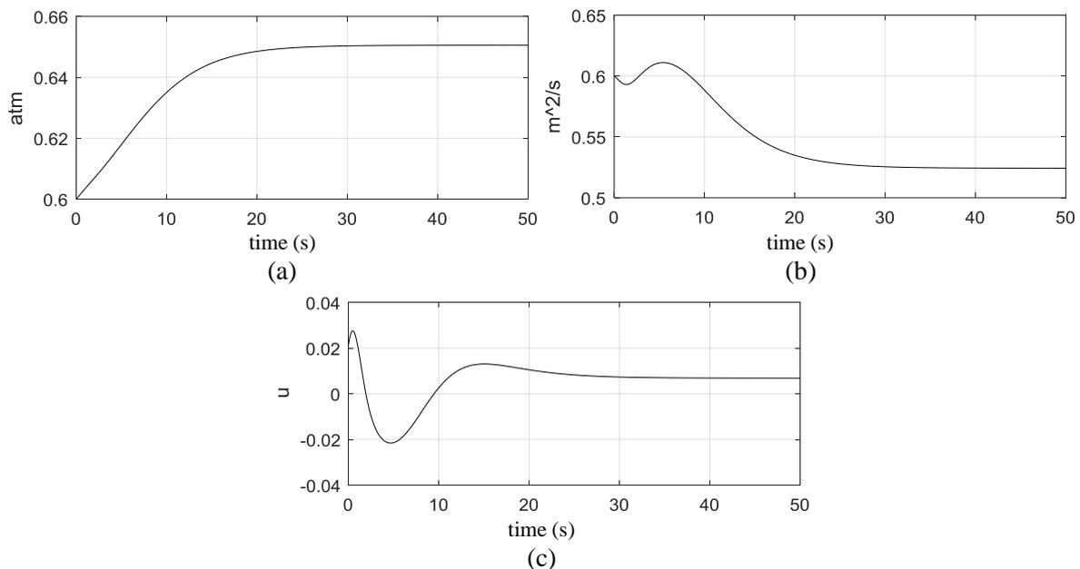
**Figure 8.** Input flow rate coefficients, output pressure and control signal with designed controller to back stepping method, (a) Changes in the output pressure coefficient, (b) Changes in the input flow rate coefficient and (c) Control signal
