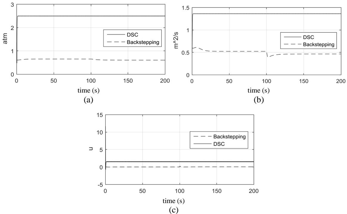
**Figure 10.** Comparison of input flow rate coefficients, output pressure and control signal in design with two control methods, a) Changes in the output pressure coefficient, b) Changes in the input flow rate coefficient and c) Control signal
