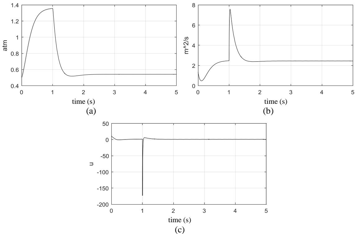
**Figure 12.** Input flow rate coefficients, output pressure and control signal with designed controller to dynamic surface method with environmental disturbance, a) Changes in the output pressure coefficient, b) Changes in the input flow rate coefficient and c) Control signal
