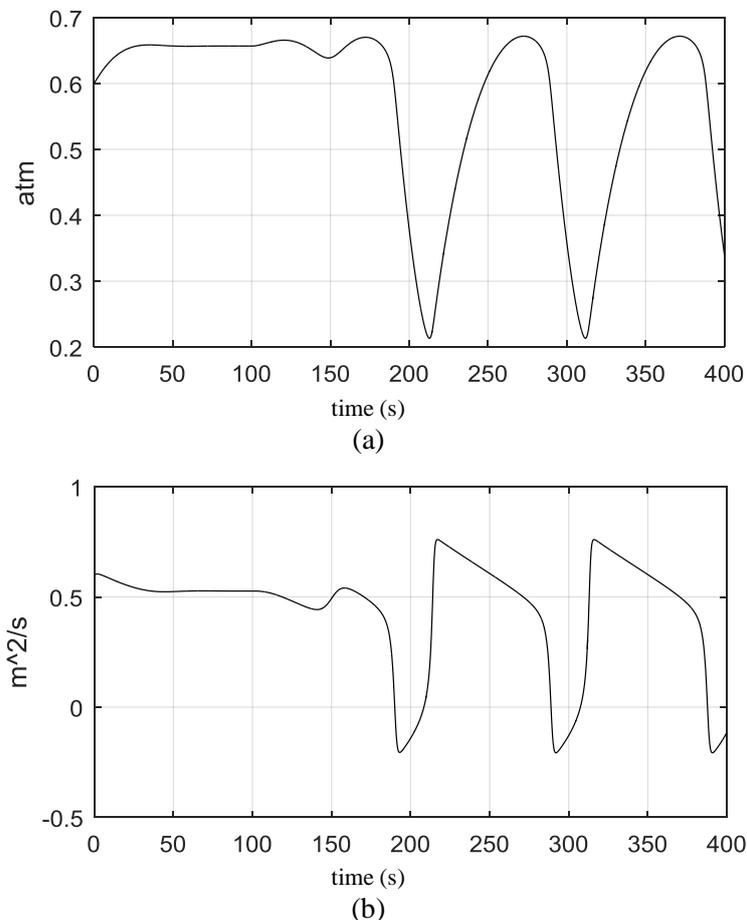
**Figure 7.** Input flow rate coefficients and output pressure without controller, (a) Changes in output pressure coefficient without controller and (b) Changes in the input flow rate coefficient without controller
