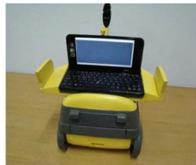
Figure 3. Mobile robot platform for the experiment. It is controlled with 1.88 GHz atom microprocessor, 2 GB RAM, 8-inch netbook computer
