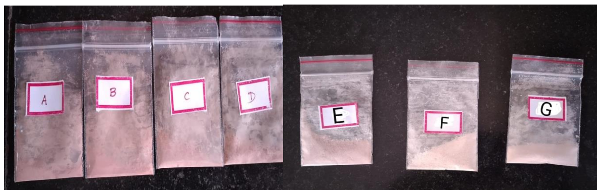
Figure 1. Pink colour formation of ZnO samples with increase in Urea
