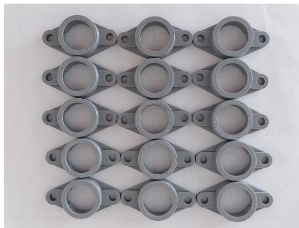
Figure 1. UCFL series roller bearings fabricated by FDM
