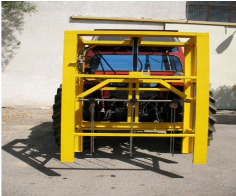
Figure 3. The tractor-mounted soil cone penetrometer for collecting cone index data in the experiment
