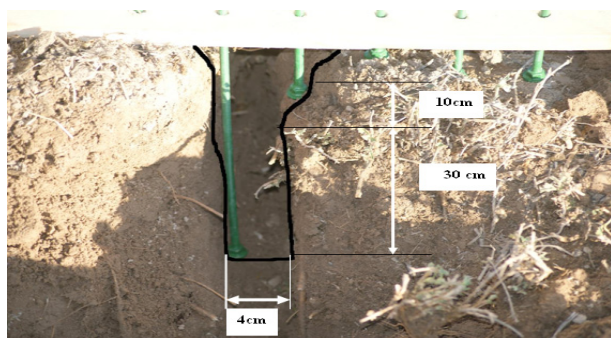
Figure 8. The cross sectional of soil disturbance perpendicular to the direction of forward speed by the OSBSMR
