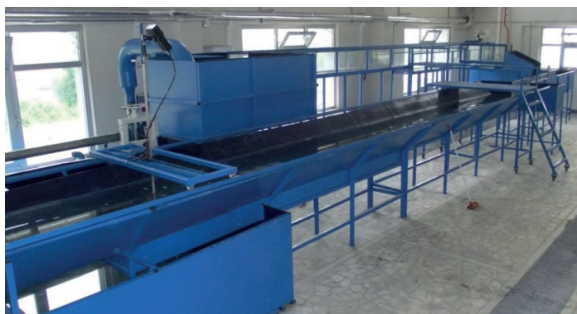
Figure 3. Open channel structure
