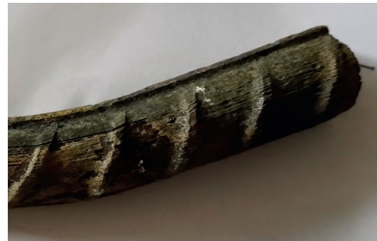
Figure 6. Surface texture of rebar after 0,5M acidic media
