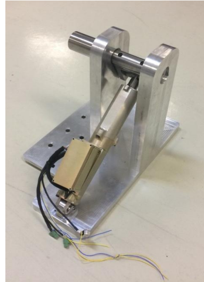
Figure 11. Fin actuating mechanism mounted on the test bench fixture.
