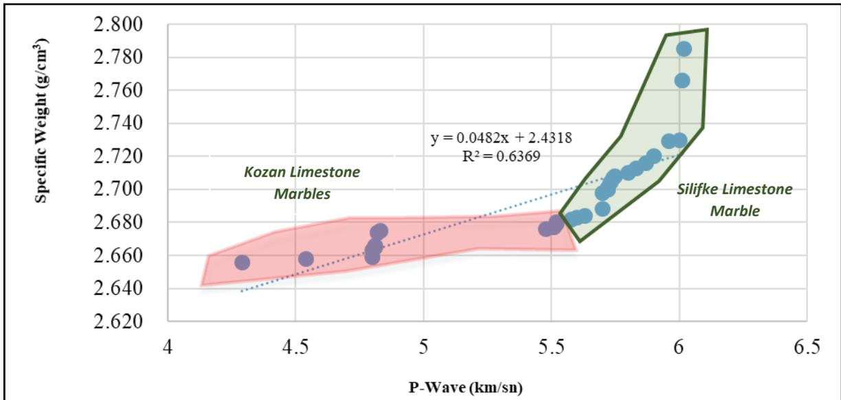
Figure 5. Correlation of P-wave velocity vs. specific weight for marbles
