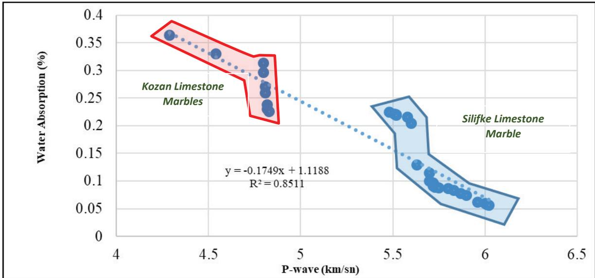
Figure 4. Correlation of P-wave velocity vs. water absorption for marbles
