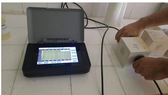
Figure 2. P wave velocity measurement of Silifke and Kozan region marbles
