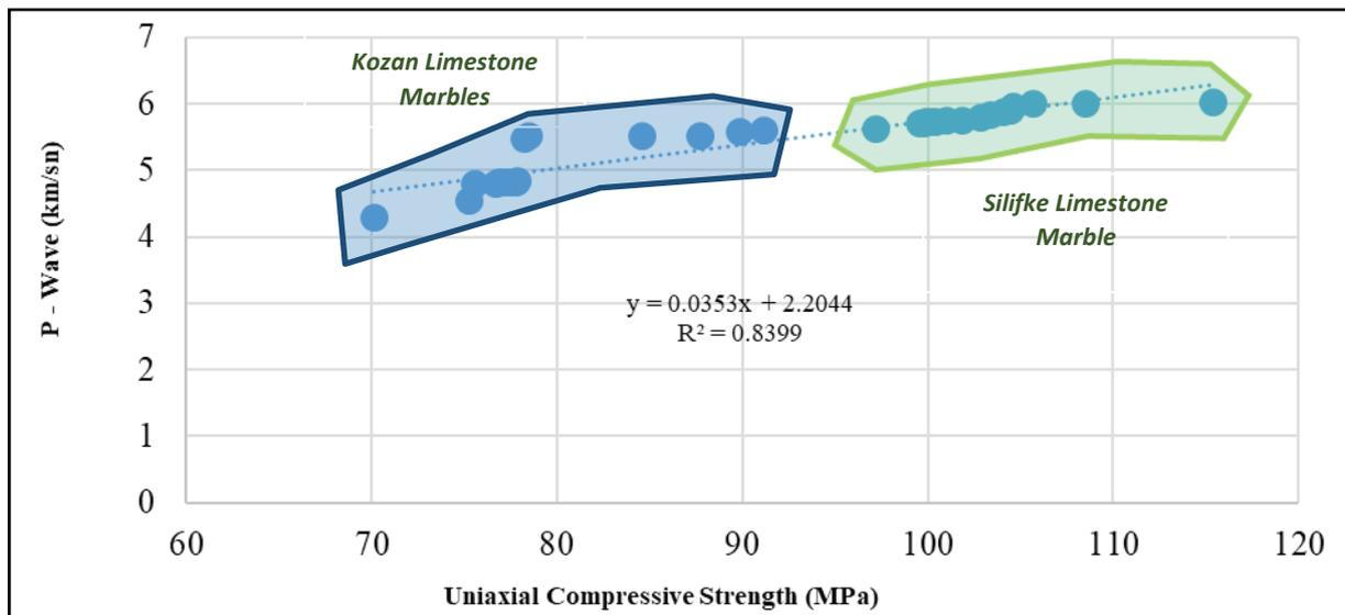
Figure 7. Correlation of P-wave velocity vs uniaxial compressive strength for marbles
