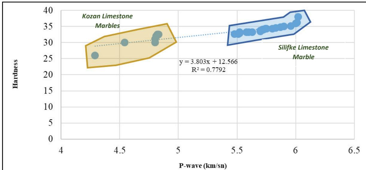
Figure 6. Correlation of P-wave velocity vs. hardness (shore) for marbles
