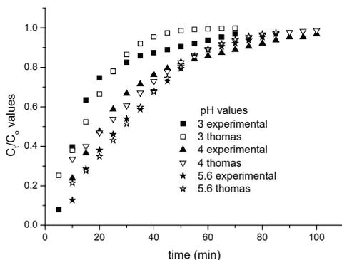
Figure 4. Breakthrough curves: the effect of different pH values on the  $\text{Cu}^{++}$  adsorption in the fixed bed.
