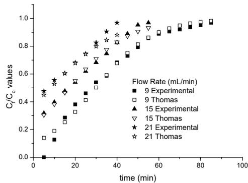
**Figure 2.** Breakthrough curves: the effect of different flow rates on Cu<sup>++</sup> adsorption in the fixed bed.
