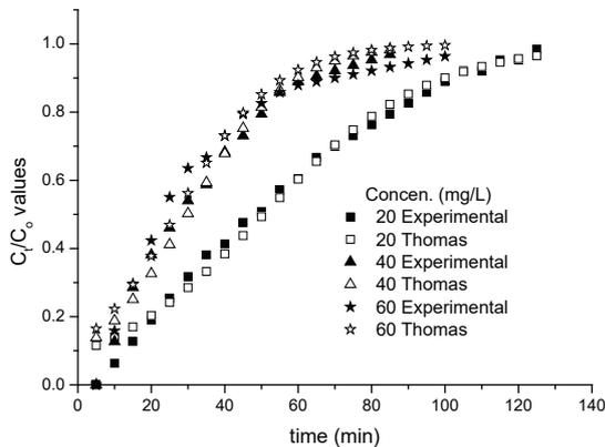
Figure 3. Breakthrough curves: the effect of influent  $\text{Cu}^{++}$  concentrations on  $\text{Cu}^{++}$  biosorption in the fixed bed.
