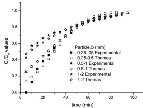
Figure 5. Breakthrough curves: the effect of different particle sizes on the  $\text{Cu}^{++}$  adsorption in the fixed bed.
