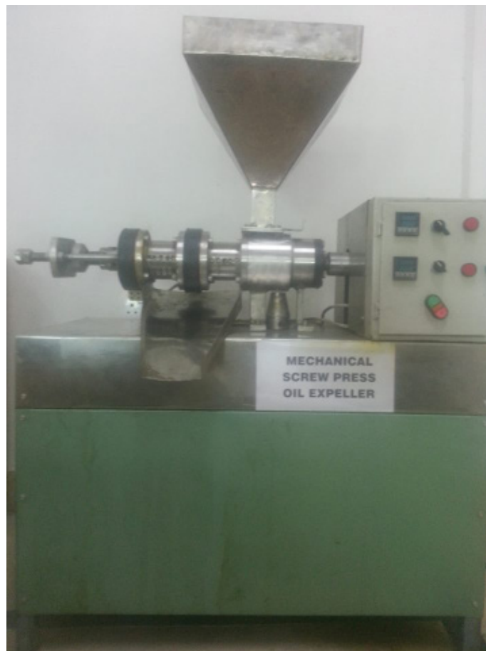
Figure 2. Extraction of Crude Oil through Mechanical Screw Oil Expeller
