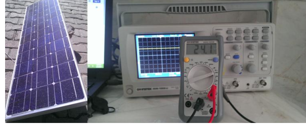
Figure 4. 24 volts and 54 watts photovoltaic arrays.
