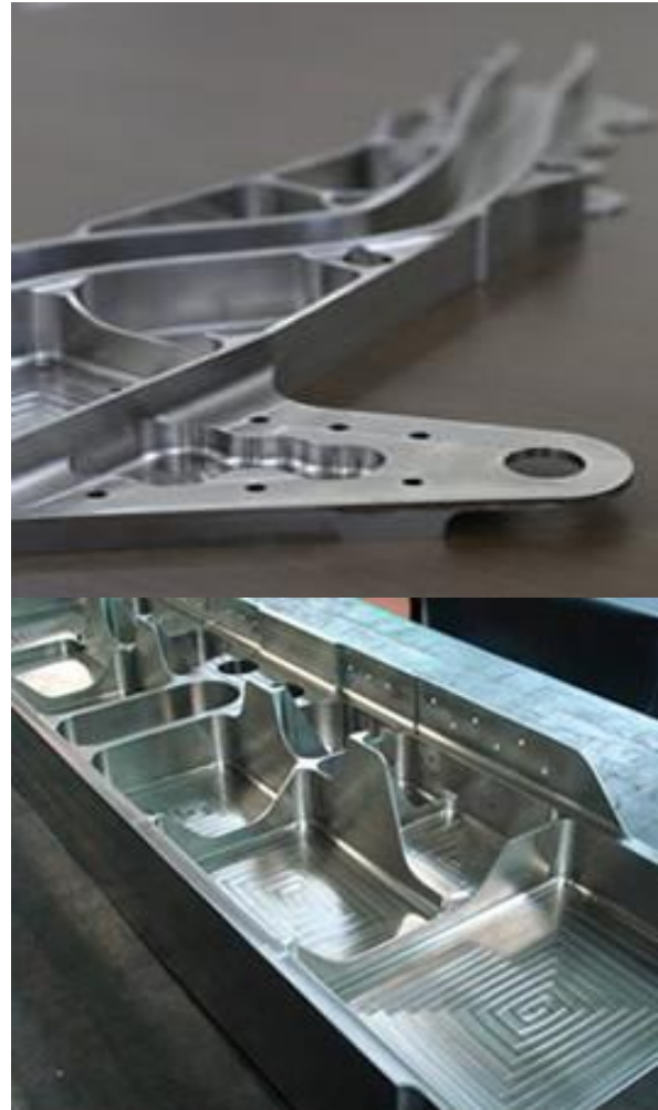
Figure 3. Ti6Al4V alloy for aircraft structure components
