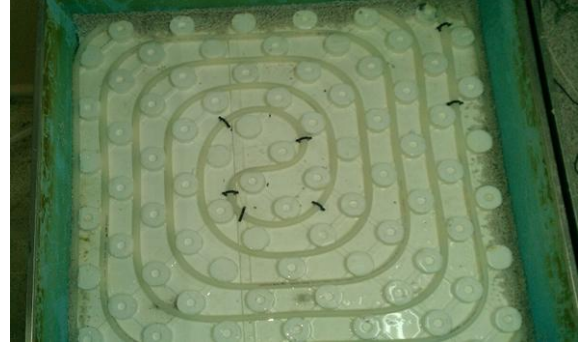
Figure 2. Placement of the floor heating pipe on the bench surface
