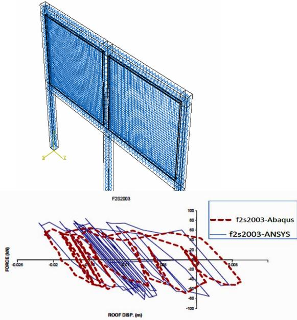
Figure2.a) Comparison of the hysteresis curve of load-displacement under acceleration b) Modeled sample according to the reference [5]
