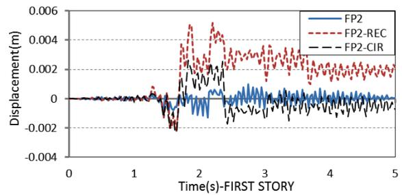
**Figure 4.** The displacement curve in terms of time for FP2, FP2-REC and FP2-CIR samples in the first story
