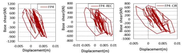
Figure 9. Hysteresiscurves of force - displacement of structure basis of FP4 ,FP4-REC and FP4-CIR
