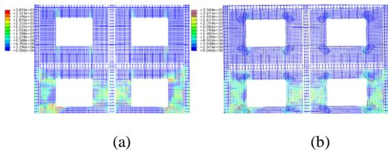
**Figure 10.** The mesh stress counter in the combined structure of FP2-REC with and without the reinforcement effect a) Without reinforcement b) With the reinforcement effect
