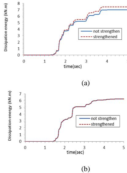
**Figure 11.** Energy dissipation in the combined structure FP2-CIR, FP2-REC with reinforcement effect a) FP2-REC b) FP2-CIR
