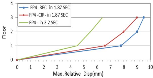
Figure 6. Comparing displacement of combined structure floors of FP4, FP4-REC, FP4-CIR
