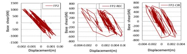
Figure 8. Hysteresis curves of force - displacement of structure basis of FP2 ,FP2-REC and FP2-CIR
