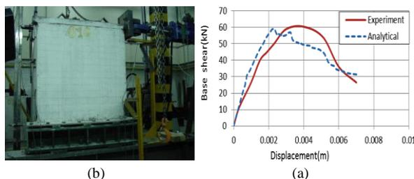
**Figure 1.** a- diagram of shear –displacement for 3D panel wall resulted from finite element analysis and the test [1] b- Location of the 3D panel wall samples and the loading system in laboratory [1]
