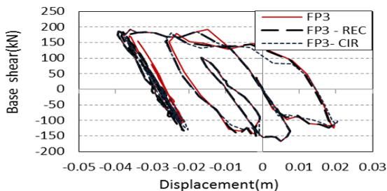
Figure 7. Hysteresis curves of force- displacement of combined structures (FP3 ,FP3-REC and FP3-CIR)
