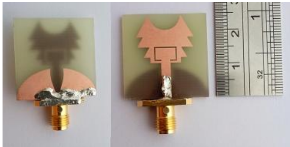
Figure 12. Photograph of the fabricated prototype, SWB antenna
