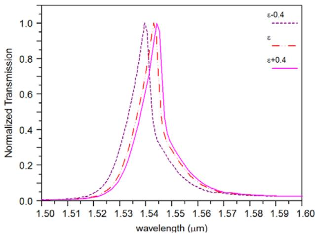
**Figure 5.** Power transmission spectra of our proposed CDF for different dielectric constants of inner rods.
