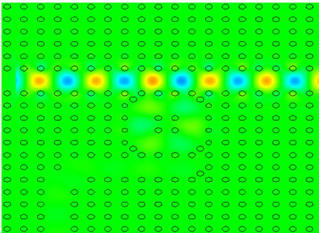
**Figure 3.** (a) Electric field intensity of the ring resonator's non-resonant wavelength at 1500nm and
