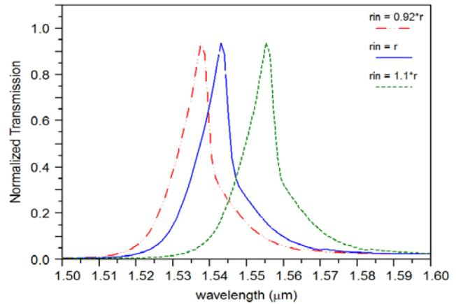
**Figure 6.** Power transmission spectra of our proposed CDF for different radius of inner rods.
