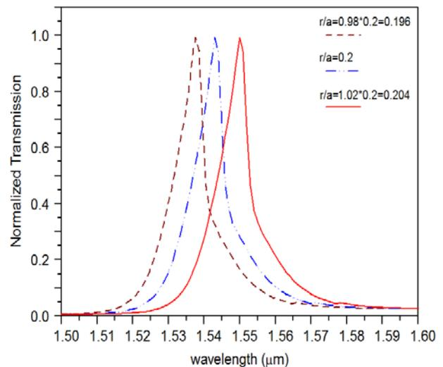
**Figure 7.** Power transmission spectra of our proposed CDF for different fill factors.
