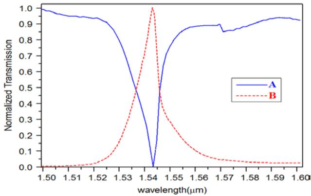
**Figure 2.** Optical power transmission characteristic of our proposed CDF in Fig. 1.
