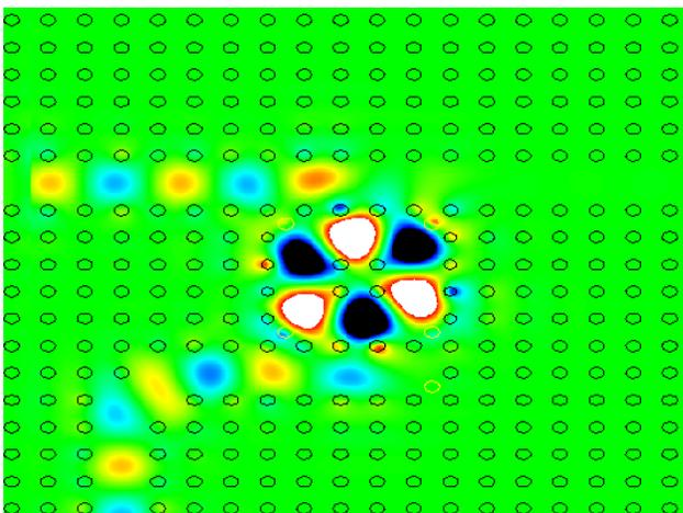
(b) electric field intensity of the ring resonator's resonant wavelength at 1543nm.
