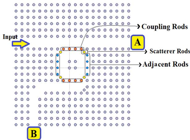
Figure 1. (a) A channel drop filter
