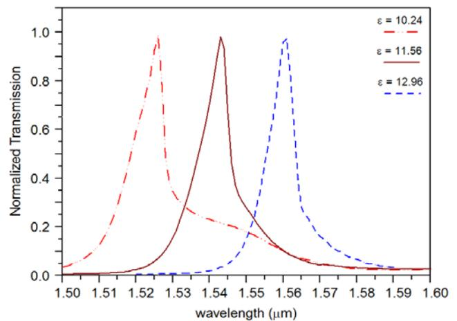
**Figure 4.** Power transmission spectra of our proposed CDF for different dielectric constants of whole rods.
