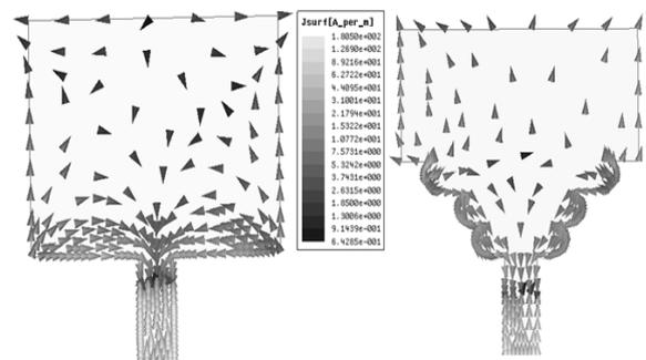
Fig.4. Simulated distribution of surface currents for Ant I and IV at 15 GHz.
