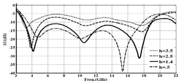
Fig. 5. Simulated return loss characteristics of the proposed antenna with different values of h (unit: mm)
