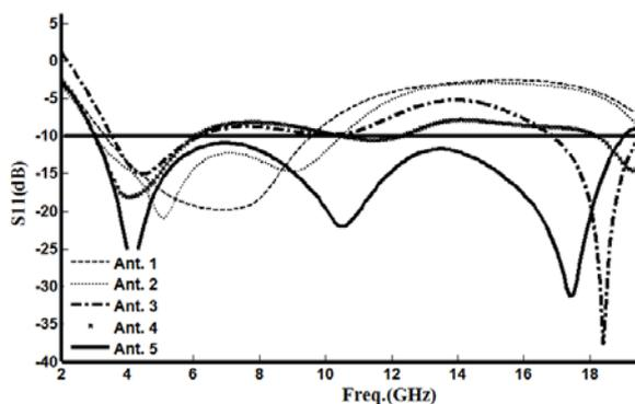
Fig.6. return loss for the antennas in Fig.2
