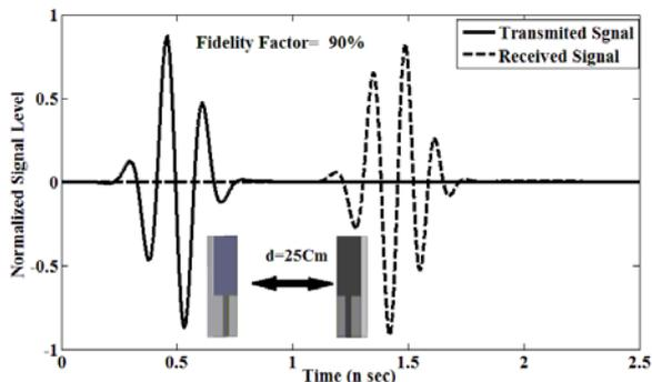
**Fig. 11.** Simulated transmitted and received pulses by the simulator CST in the position face to face
