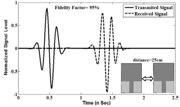
**Fig. 12.** Simulated transmitted and received pulses by the simulator CST in the position side by side.
