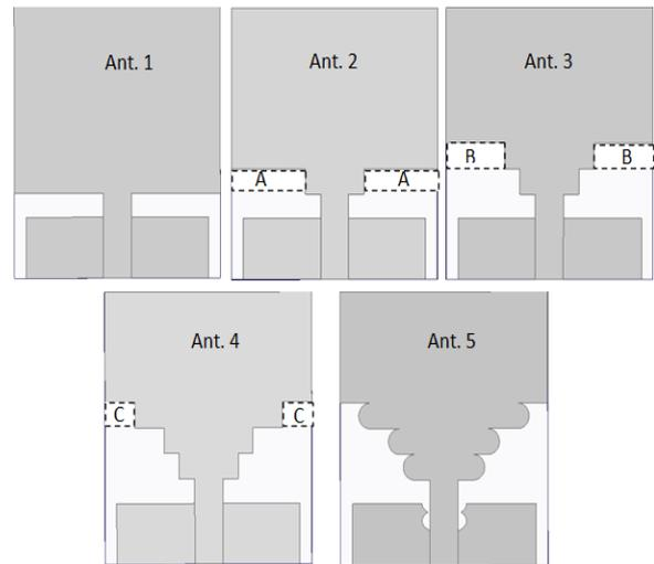
Fig.3. The configuration of the five proposed antenna
