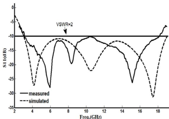
Fig.7. Measured and simulated return loss curves versus frequency for the proposed antenna
