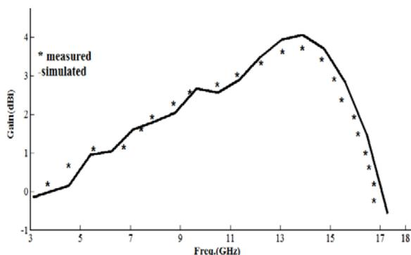
Fig.8. Measured and simulated gain of the proposed antenna
