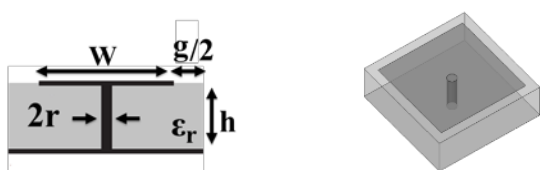
Figure 5. Mushroom-like EBG Unit Cell Parameters.
