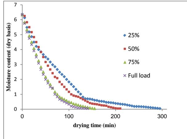
Figure 3. Variation of moisture content with drying time at different engine loads when sample thickness is 5 mm.
