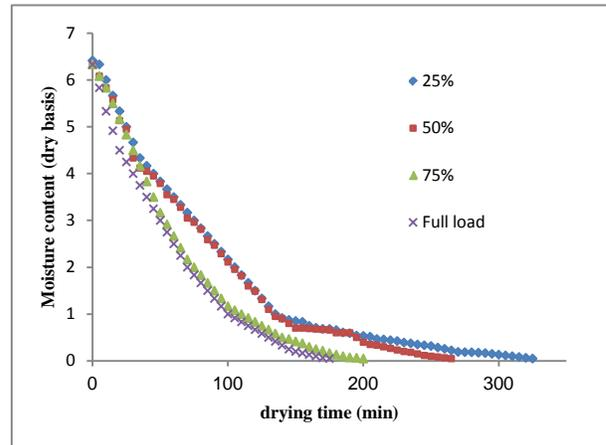
Figure 4. Variation of moisture content with drying time at different engine loads when sample thickness is 7 mm.
