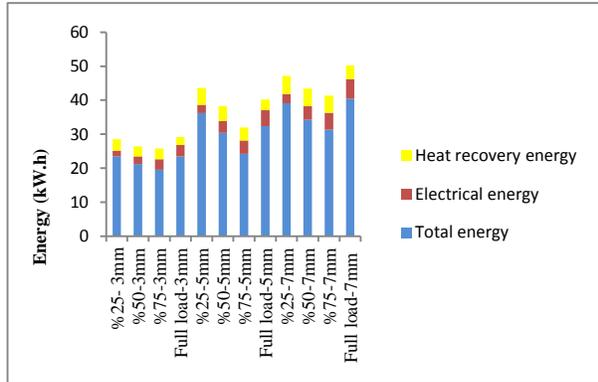
Figure 5. Total and useful energy consumption at different thickness and engine loads.
