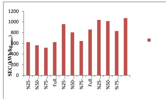
Figure 8. Specific energy consumption of drying at different thickness and engine loads.
