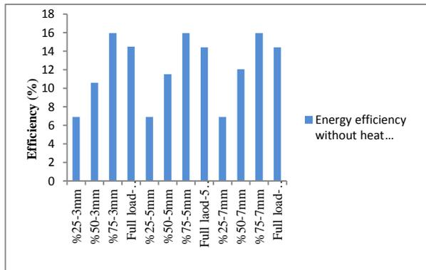
Figure 6. Energy efficiency without heat recovery at different thickness and engine loads.
