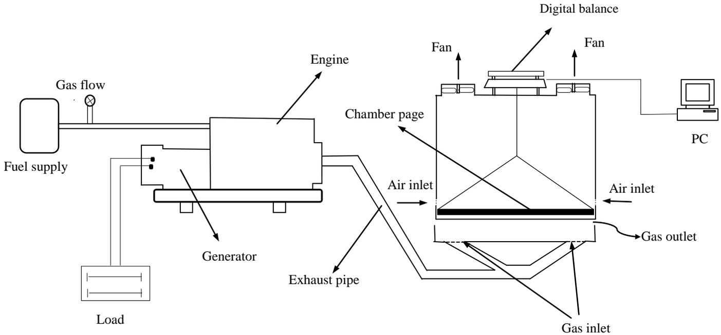
Figur1. Schematic diagram of the drying equipment
