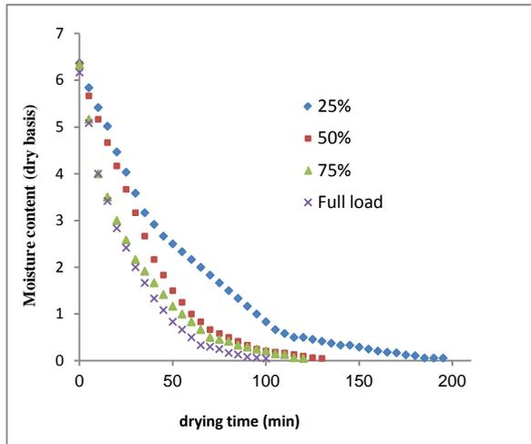
Figure 2. Variation of moisture content with drying time at different engine loads when sample thickness is 3 mm.
