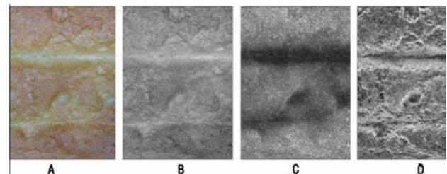
Figure 3. Example of converted image; A: sample of cut photo B: L\* component of image C: a\* component of image D: b\* component of image
