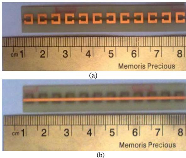
Figure 2. fabricated BBSCMM-SR (a) top view of (b) bottom view.
