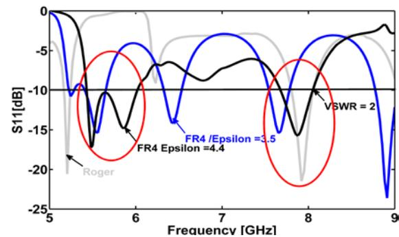
Figure 6. Return loss plot for Antenna with different Substrates
