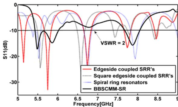
Figure 5. Return loss plot for Antenna with different Methods
