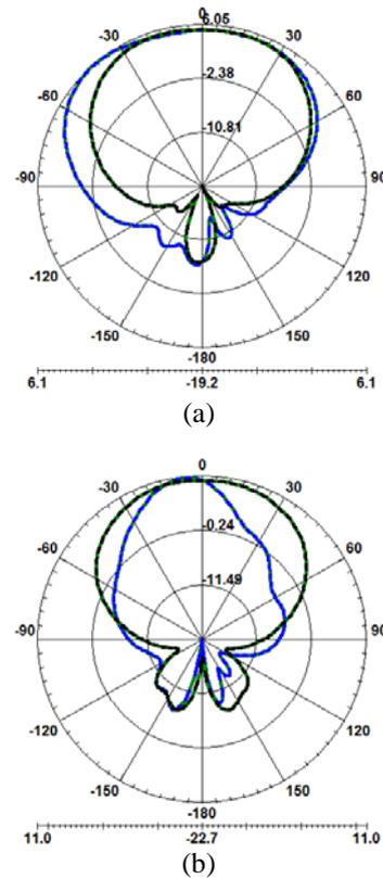
Figure 4. Measured E-plane and H-plane of antenna with 6 unit cells in (a) 5.48GHz (b) 5.88GHz
