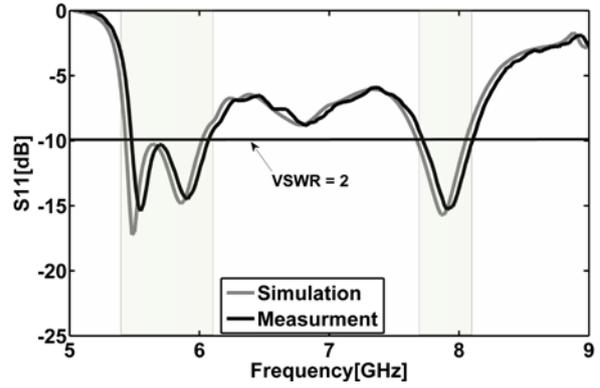
Figure 3. Measured and simulated  $S_{11}$  plot for Antenna with 6 unit cells for FR4 substrate.
