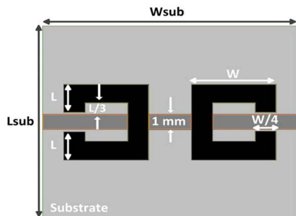
Figure 1. Unit cell of new metamaterial
