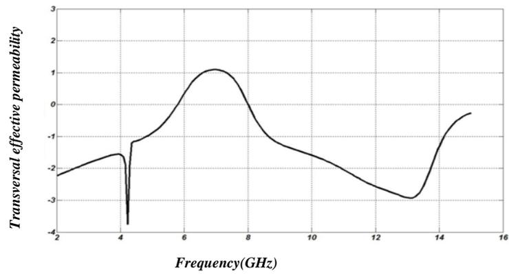
Figure 4. Transversal effective permeability of omega shaped metamaterial
