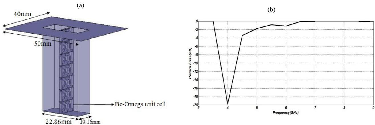
Figure 6. (a) Waveguide antenna with metamaterial structure (b) Return loss diagram
