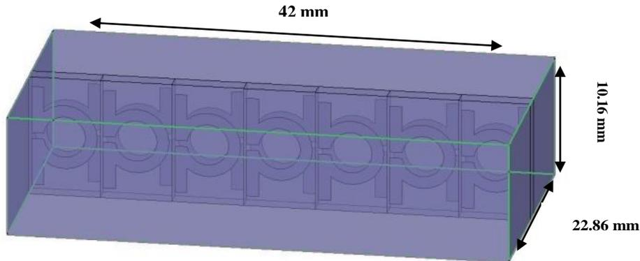
Figure 3. Schematic of filling waveguide with metamaterial
