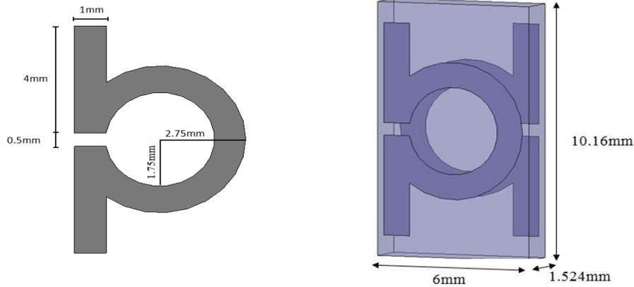
Figure 2. (a) Copper ring (b) unit cell of metamaterial structure
