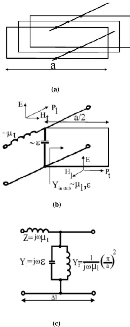
**Figure 1.** (a) Transmission line representation of a rectangular waveguide (b) Inductance and capacitance model (c) Equivalent circuit of a waveguide filled with uniaxial metamaterial [2].
