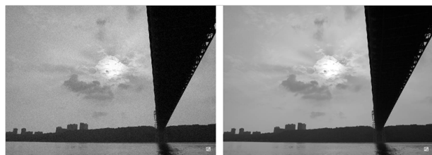
Fig.5. Correction with 5% gain and 10% bias FPN noise. (left) Before correction whit MSE = 33.88. (right) After correction with MSE = 4.95.
