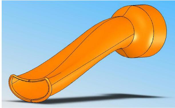
Fig.2. Schematic of the air intake.
