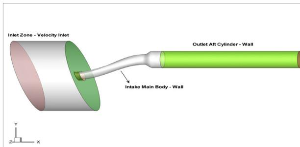
Fig.3. Final 3-D model and boundary definition.
