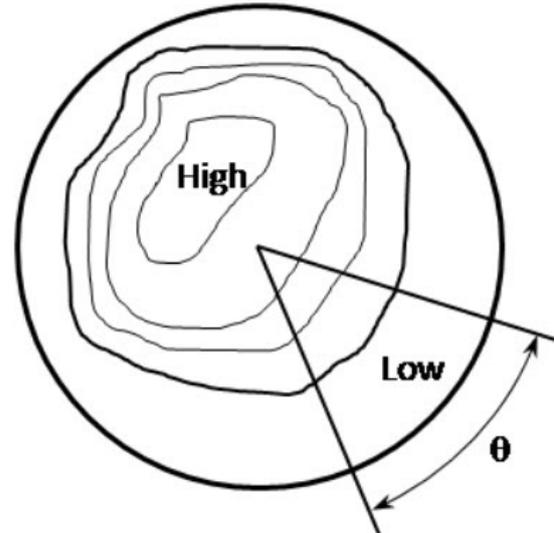
Fig.1. Illustration of total pressure contours to define distortion coefficient [3].
