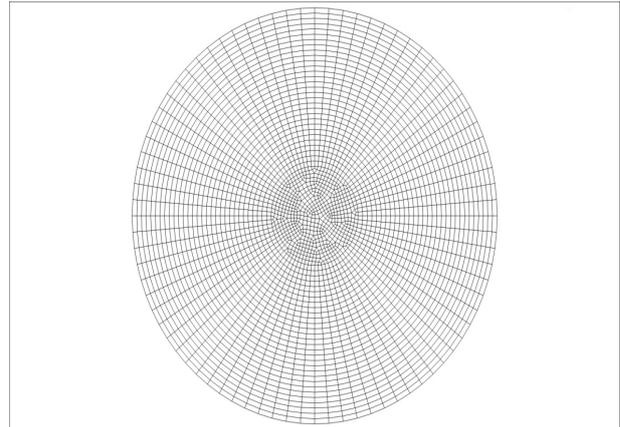
Fig.4. Quad mesh of outlet zone with the inner Pave and outer Mapped grid.
