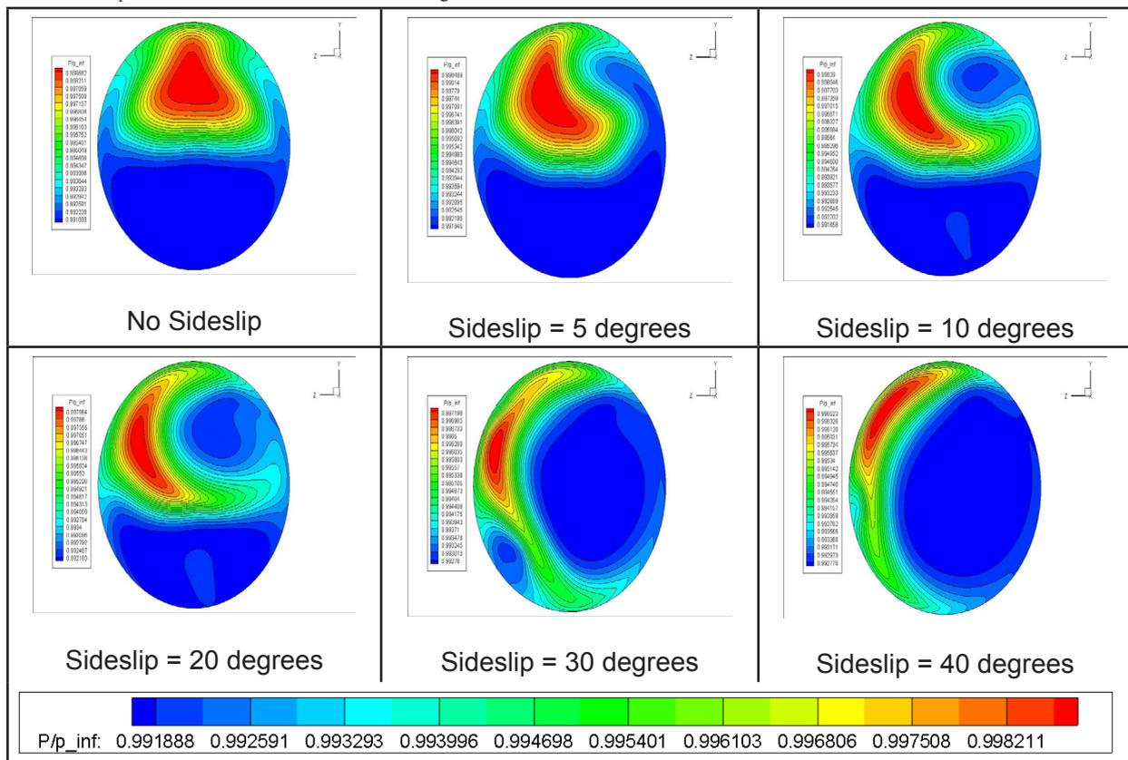
Table.5. Total pressure distribution at AIP in steep angle climb condition.
