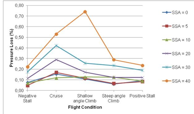
Fig.7. Total pressure loss at AIP in different flight conditions at Sideslip angles.
