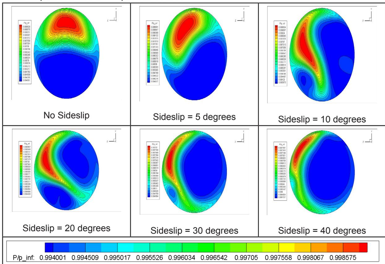
The obtained values specified in Figure 7, total pressure recovery is a bit sensitive to side slip angle changes. Therefore it is concluded that this air intake is properly designed in terms of performance at side slip condition.
