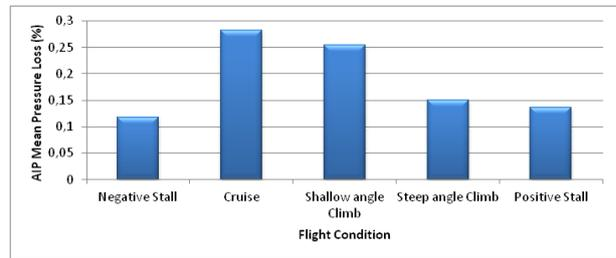
Fig.6. Mean total pressure loss at AIP in different flight conditions.
