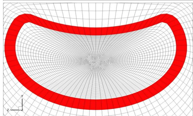
Fig.5. Quad mesh of Pave-Map of inlet zone.
