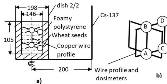
Figure 1. Geometry and irradiation technic
