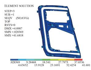
Figure 16. Equivalent Stress distribution from Finite Element Random Vibration in X axis with material data obtained from test coupon cut from Bezel.
