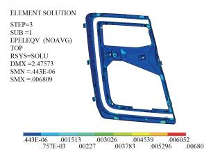
**Figure 10.** Equivalent Strain distribution from Finite Element Random Vibration in Y axis with material data from dog bone type tensile test specimen.
