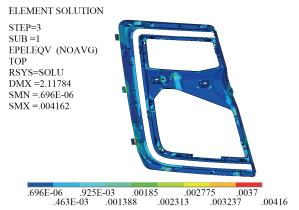
**Figure 9.** Equivalent Strain distribution from Finite Element Random Vibration in X axis with material data from dog bone type tensile test specimen.
