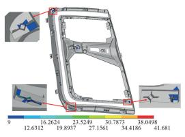
**Figure 17.** Failure definition through Finite Element Random Vibration in X axis with restricting stress values between yield stress and maximum stress from finite element simulation.
