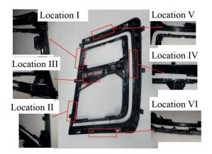
Figure 5. Locations of test coupon cut from Bezel with different travel distance.
