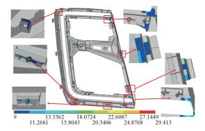
**Figure 19.** Failure definition through Finite Element Random Vibration in Y axis with restricting stress values between yield stress and maximum stress from finite element simulation.
