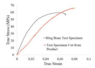
Figure 3. Material characteristics for PC from dog bone test specimen and test coupon cut from product.
