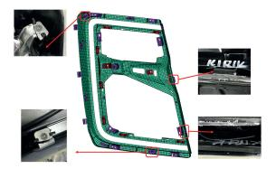
Figure 14. Failure after vibration test of Bezel with 180 MPa of injection pressure and 70 MPa holding pressure.
