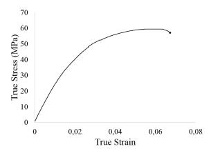
Figure 2. Material tensile test data for PC material at 1 mm/ min.
