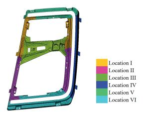
Figure 15. Material mapping of Bezel considering travel distance effect on mechanical performance.
