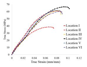
**Figure 6.** Travel distance effect on mechanical performance predicted through tensile tests.
