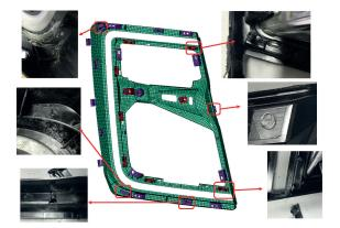
Figure 13. Failure after vibration test of Bezel with 180 MPa of injection pressure and 50 MPa holding pressure.
