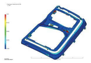
Figure 12. Fraction of solidification in Bezel after Injection moulding.
