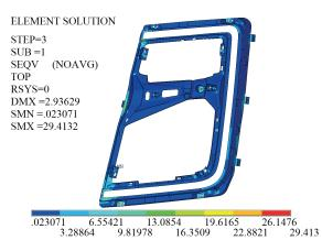
Figure 18. Equivalent Stress distribution from Finite Element Random Vibration in Y axis with material data obtained from test coupon cut from Bezel
