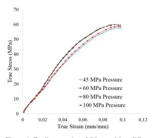
Figure 4. Tensile properties of PC material at different holding pressures.
