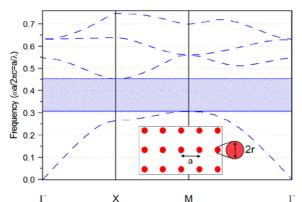
**Figure 1.** Band diagram of the PC perfect lattice calculated in TM polarization mode by PWE method, this PBG is maxima for filing ratio r/a=0.17.
