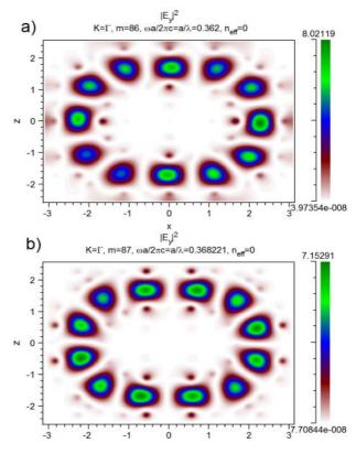
Figure 6. The main resonant modes of the all circular PCRTR with the normalized frequency (a) 0.362 and (b) 0.368.
