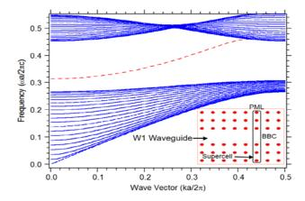
Figure 2.  $W_1$  waveguide dispersion curve, calculated by PWE method for both PC perfect lattice and PC with line defect (waveguide).
