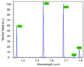
Figure 5. Resonant modes of the race track resonator in the bandgap region calculated using FDTD method. M1-M5 are the PCRTR resonance modes.
