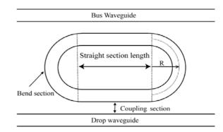
Figure 3. Schematic design of a single ring racetrack resonator. The race track consists of a straight section and the bends.
