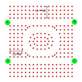
Figure 7. Three dimensional view of the designed filter. The coupling section is  $L_C=4a$  in the all directions of the PCRTR.
