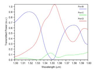
Figure 8. Transmission spectral response of the proposed CDFcalculated using FDTD method. The center wavelenght of this filter is  $\lambda$ =1.55 $\mu$ m.
