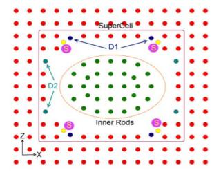
**Figure 4.** Demonstration of the designed PCRTR and its selected supercell which is used to calculate the resonant modes. D1, D2and S are 12 introduced defects in the PCRTR to improve its performance.
